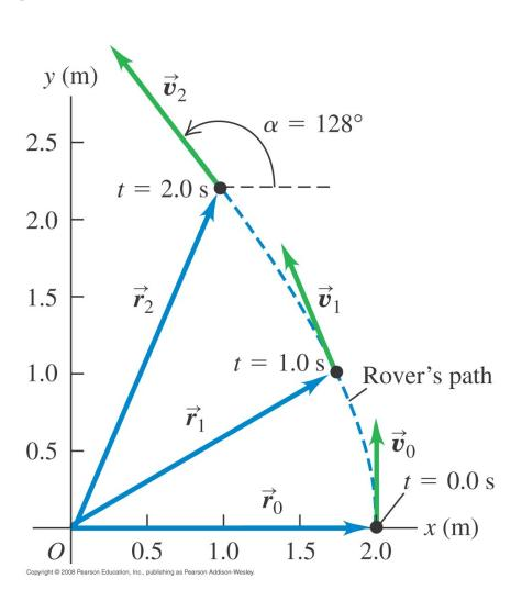
This illustration shows the path of a robotic vehicle, or rover. What is the direction of the rover's average acceleration vector for the time interval from t = 0.0 s to t = 2.0 s?
